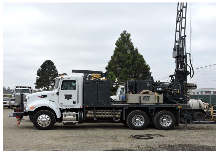
Boring truck rig that will take soil samples.
